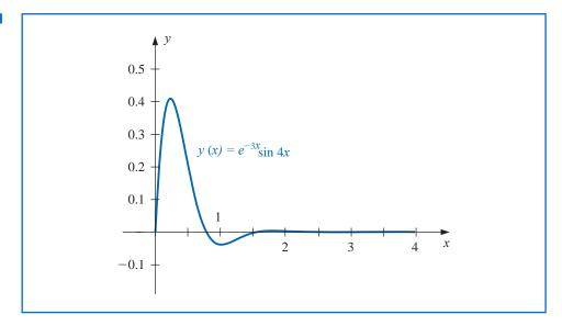
Suppose that we need the integral of y(x) on [0,4]. The graph indicates that the integral on [3,4] must be very close to 0, and on [2,3] would also not be expected to be large. However, on [0,2] there is significant variation of the function and it is not at all clear what the integral is on this interval. This is an example of a situation where composite integration would be inappropriate. A very low order method could be used on [2,4], but a higher-order method would be necessary on [0,2].
