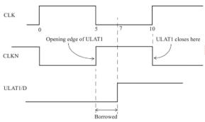
(b) Clock and data waveforms for 7ns data path.
