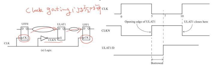
(b) Clock and data waveforms for 7ns data path.
