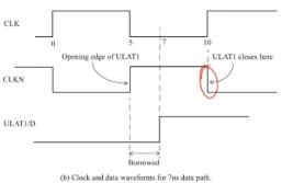
Endpoint: ULAT1 (positive level-sensitive latch clocked by CLK') Path Group: CLK Path Type: max Point Incr Path clock CLK (rise edge) 0.00 0.00 0.00 0.00 clock source latency 0.00 r 0.00 clk (in) UFF0/CK (DF ) 0.00 0.00 r UFF0/Q (DF ) 0.12 0.12 r UBUF0/Z (BUFF 6.65 6.77 r UBUF1/Z (BUFF 4.33 11.10 r UBUF2/Z (BUFF 11.17 r 0.07 (11.17) r ULAT1/D (LH ) 0.00 11.17 data arrival time
