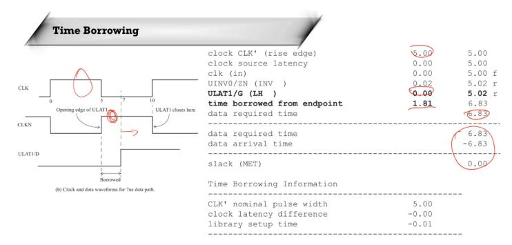
In this case, since the data becomes available while the latch is transparent, the required delay of 1.81ns is borrowed from the subsequent path and the timing is still met.
