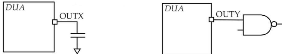
Figure 7-31 Capacitive load on output port.
