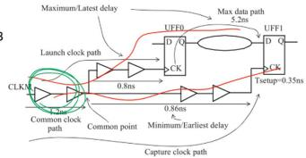
Applying the OCV derating has increased the minimum clock period from 5.49ns to 6.81 lns for this example design.
