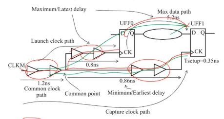
The worst condition for setup check occurs when the <u>launch clock path and the data path have the OCV</u> conditions which result in the <u>largest delays</u>, while the capture clock path has the OCV conditions which result in the <u>smallest delays</u>.
