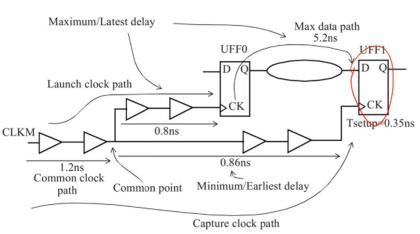
考虑OCV的影响,launch path delay \* 1.2,capture path delay \* 0.9,Tsetup \* 1.1,需 要的最小周期为7.171ns
