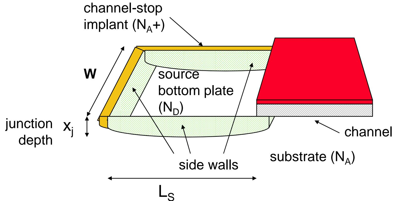
$$\begin{aligned} C_{\text{diff}} &= C_{\text{bp}} + C_{\text{sw}} = C_j \text{ AREA} + C_{j\text{sw}} \text{ PERIMETER} \\ &= C_j L_S W + C_{j\text{sw}} (2L_S + W) \end{aligned}$$
